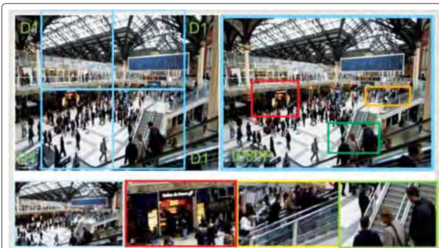
Figure 1: Boxes on the above image shows difference in 4 x D1 images vs. 1 x 1080P HD image and how 'areas' of the image can be zoomed in on from any terminal
